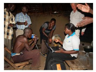
Measurement of particulate matter (PM) with the DustTrak II (from TSI) is not that easy. We have a technical problem as the batteries don't last 24 hours. Furthermore people in a household are often scared of the device. One cleaned it every hour and another didn't dare to cook anymore.
