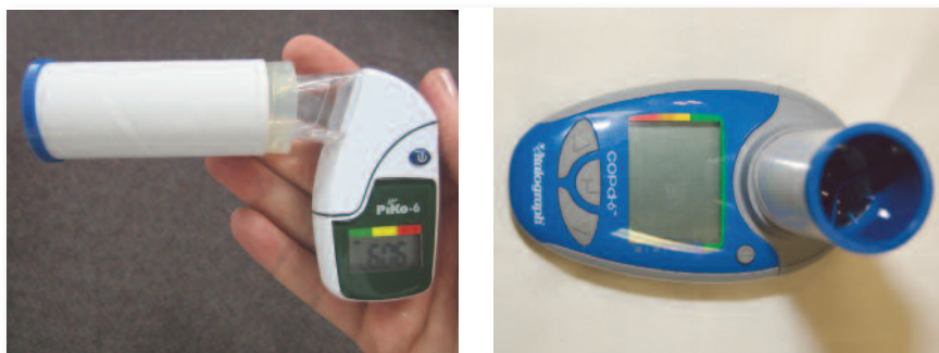
Figures 2a and b. Digital COPD screening devices. a (left). PiKo-6, with mouthpiece adaptor and one-way valved cardboard mouthpiece attached. b (right). Vitalograph COPD-6, with one-way valve mouthpiece attached.
